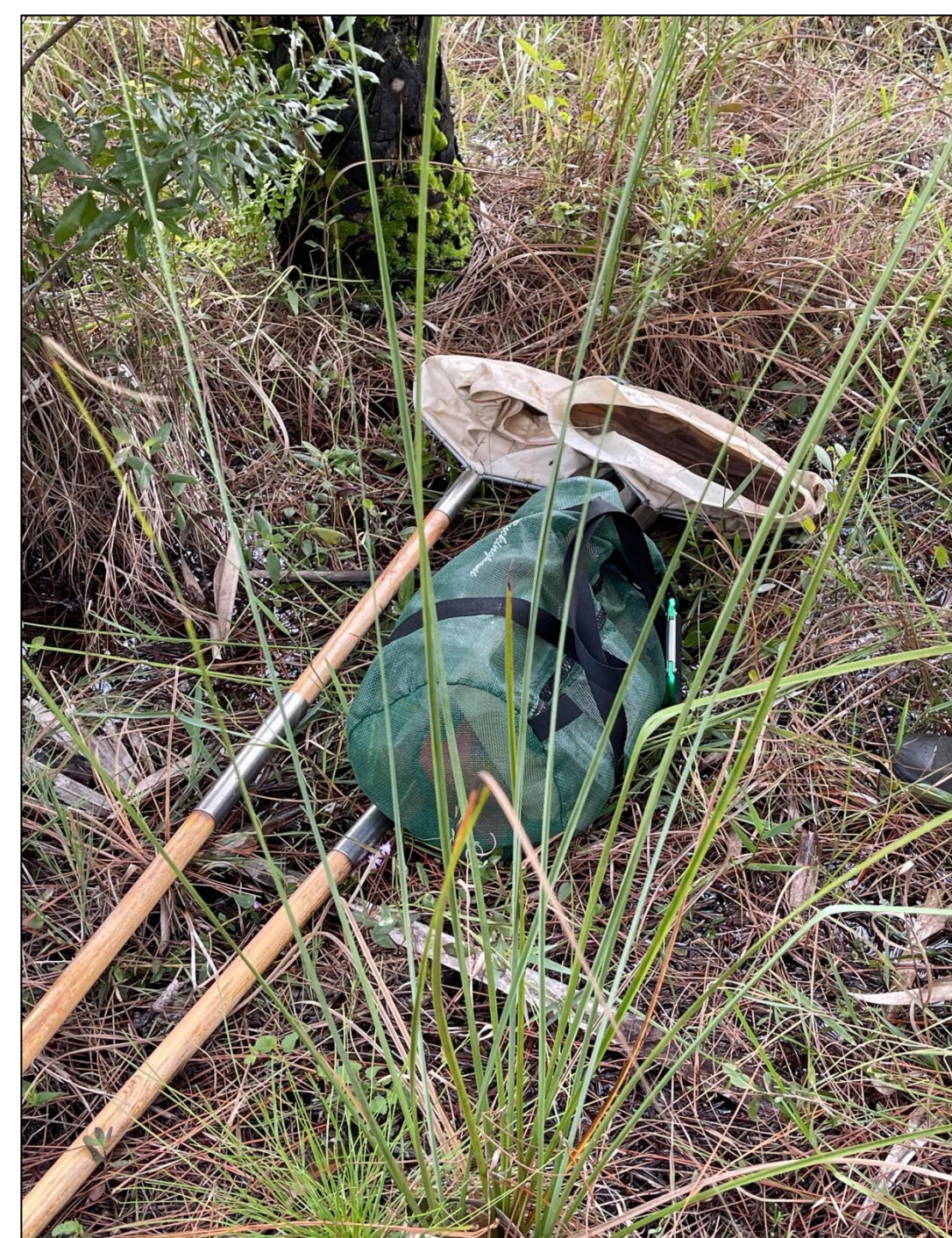
D-frame dip nets for aquatic macroinvertebrate sampling
